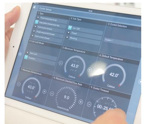
Each Intelligent Care tap can be operated through Rada's app and programmed independently to meet unique requirements. Everything from run times and temperatures, right through to hygiene measures such as duty flushing, can be programmed and monitored remotely.
