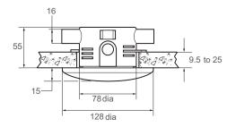
**Specify as: Mono-Control System MC126 (1.1495.013)** Each group of urinal bowls to be served by one Rada Mono-Control System MC126 ceiling mounted flow control. Complete with concealed passive infra-red sensor, control module and ½" solenoid valve with isolator and filter.
