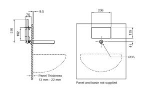
Dimensions shown are the finished product dimensions and should not be used as a guide for cutting panels.
