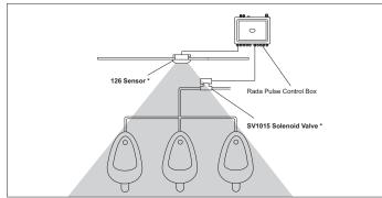
Only the Sensor and Solenoid are supplied with this operating system as indicated \*
