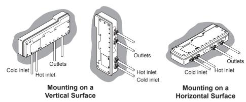
**Note!** If the DMV is installed in a different orientation to those shown above, it may cause the DMV to malfunction e.g. cause airlocks, water ingress and could effect the thermal performance of the DMV.
