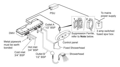
**Note!** The Data Cable must be placed through the Suppression Ferrite and then looped around the cover. The Suppression Ferrite must be fitted as close to the Control Panel as possible.
