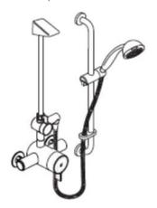
**Concealed Model:** This diverter is designed to be installed on the outlet of the Rada V12 Concealed Mixer. A flow regulator (6 and 9 l/min supplied with the Rada V12 Mixer) can be fitted to the right angled connector (RAC) if required.
